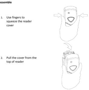
Note: DO NOT use a screw driver or other implement to remove cover. Incorrect removal of cover may damage the LED and void the warranty.
