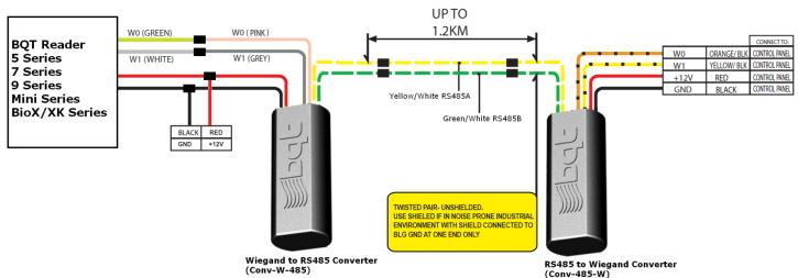
W-485 marked converter is connected to reader
