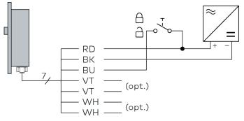
When in Fail Secure configuration, applying positive voltage to the control wire triggers the YD30D to unlock (active-low locking signal). In the event of a power cut, the YD30D will remain locked.
