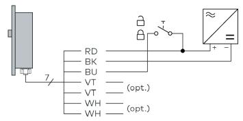
When in Fail Safe configuration, applying positive voltage to the control wire triggers the YD30D to lock (active-high locking signal). In the event of a power cut, the YD30D will unlock.
