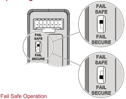
Assume the lock is installed, wired, and set to fail safe. The door is open and the positive supply voltage is applied to the **BLUE** wire. As the door closes the YD30S senses the door approaching and activates the bolt pin to pull the door into alignment. The Bolt Position and Door Position monitors will have changed to closed contact state as the door is closed and secured.
